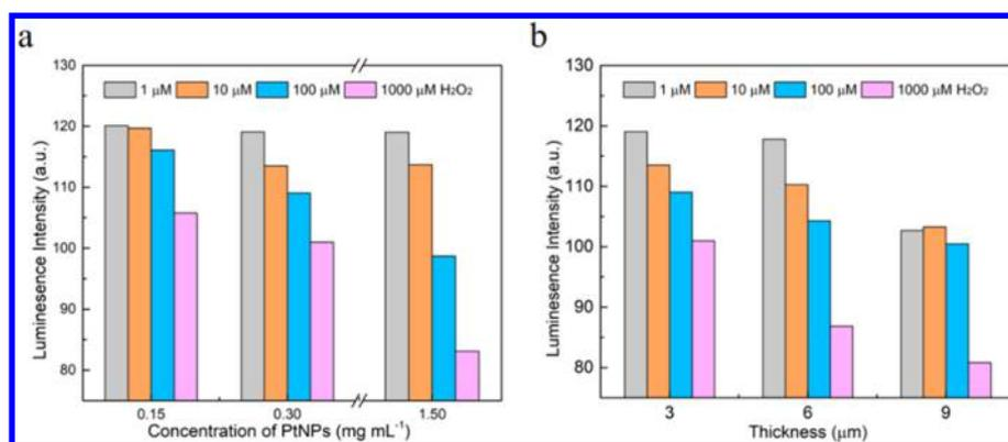
**Figure 1.** Response of sensor films with different concentration of PtNPs (a) and thickness of catalyst layer (b) at different concentrations of H<sub>2</sub>O<sub>2</sub> marked in color. The sensor performance was improved by increasing the concentration of PtNPs and using thicker film. However, the sensor performance will decrease when the thickness of catalyst layer reach to 9.0 μm.
