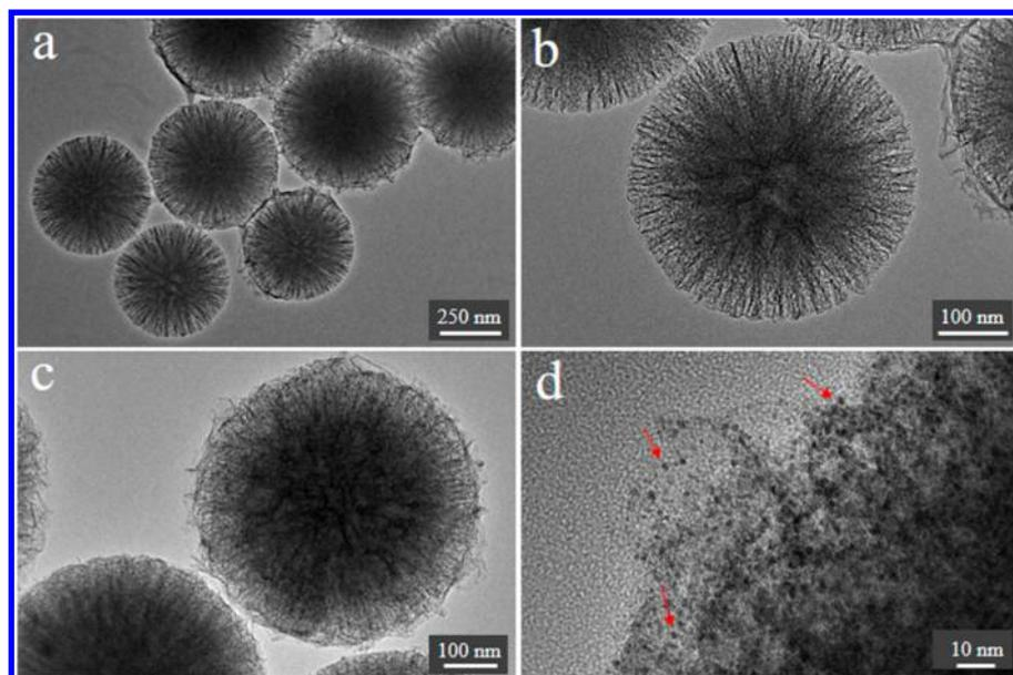
**Figure 2.** TEM images of bare KCC-1 particles (a, b) and PtNPs-decorated KCC-1 particles (c, d) with low (left) and high (right) magnification. The V-shape pores can be clearly seen in the magnified pictures, and PtNPs (shown with red arrow) are uniformly distributed inside the pores (d).
