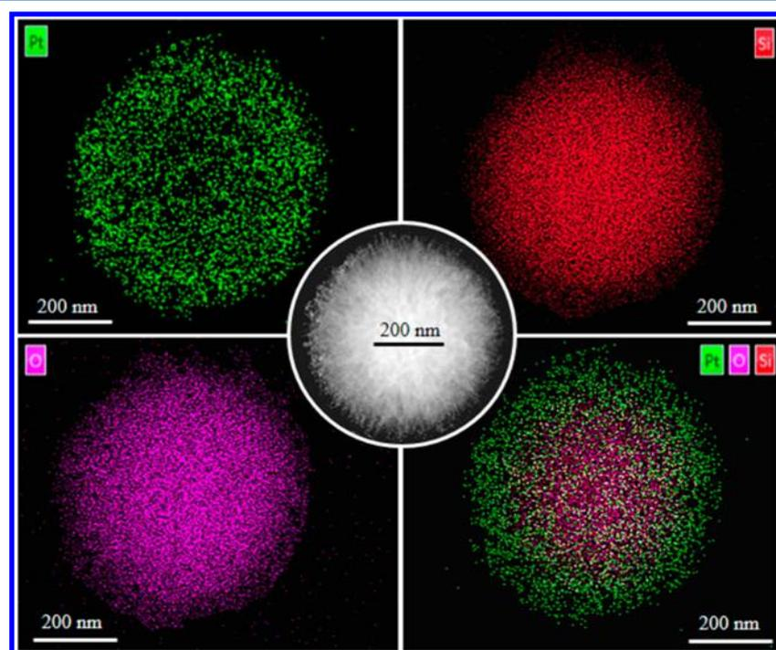
**Figure 3.** EDX element mapping images of the elements Pt, Si, and O in a single KCC-1-PEI/PtNPs. From the Pt (green color) and Si (red color) mapping images, it is clear that PtNPs are uniformly distributed throughout the entire KCC-1 particle.
