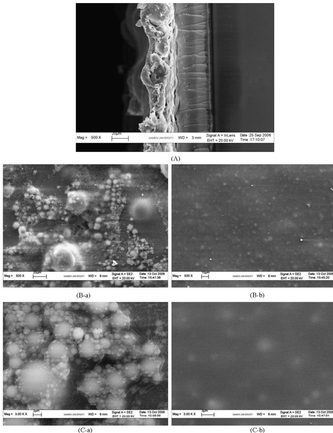
Fig. 2. Scanning electron micrograph of glucose sensor: (A) section and comparison of (a) with- and (b) without-immobilized glucose oxidase at (B) low and (C) high magnification.
