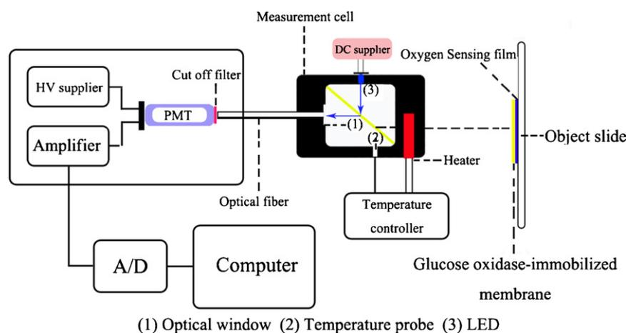
Fig. 1. Setup for the optical sensing measurement of glucose.
