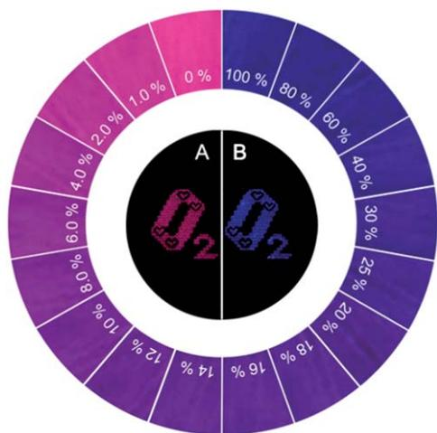
**Fig. 2** Apparent colours of the chameleon cloth at different oxygen concentrations. (A) real picture of the chameleon cloth marker exposed in an oxygen-free environment; (B) real picture of the chameleon cloth marker under UV excitation in pure oxygen.
