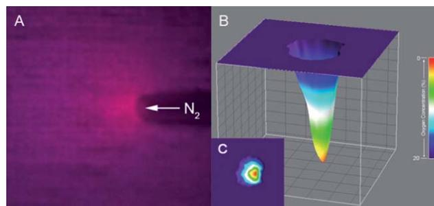
**Fig. 1** (A) Apparent colour of the prepared chameleon cloth exposed to a flow of nitrogen in air; (B) Quantitative imaging of oxygen distribution using photographic technique<sup>12–15</sup> (corresponding to Fig. 1(A)); (C) Top-view of Figure 1(B) shows the oxygen deficiency range and oxygen-free area.
