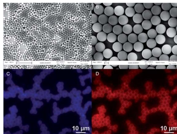
**Fig. 3** Scanning electron microscope images of the oxygen-sensitive polystyrene microparticles at low (A) and high (B) magnification; and fluorescence microscope images of the oxygen-sensitive polystyrene particles: (C) the blue emission of the stilbene dye, (D) the red emission of the PtOEP oxygen probe in air.
