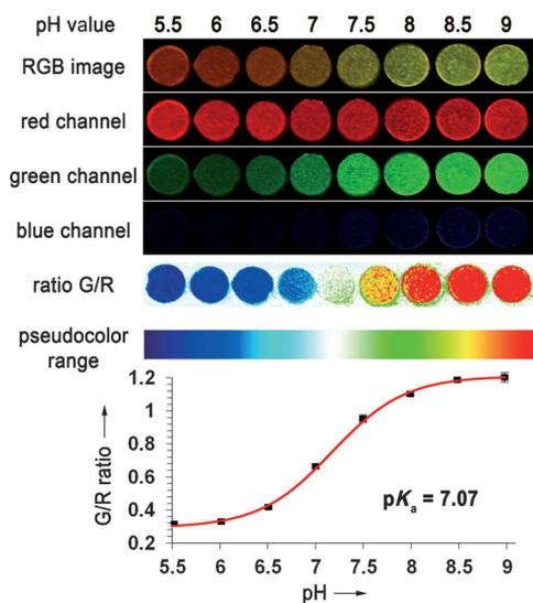
**Figure 2.** Optical response of the pH-sensitive agarose Petri dish, see text for details.
