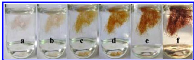
**Figure 5.** Response time of a carboxymethyl–dithiocarbamate modified polyacrylonitrile fiber for  $Ag^+$  ( $1 \times 10^{-2}$  mol/L) at (a) 0 s, (b) 10 s, (c) 2 min, (d) 10 min, (e) 1 h, and (f) 24 h at pH 5.5. (Reprinted from *J. Hazard. Mater.* Vol. 297, Xing, X.; Yang, H.; Tao, M.; Zhang, W. An overwhelmingly selective colorimetric sensor for  $Ag(I)$  using a simple modified polyacrylonitrile fiber, pp. 207–216 (ref 169). Copyright 2015, with permission from Elsevier).
